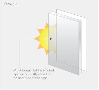
Opaque is a light-blocking layer that creates a fully opaque panel and comes in 13 neutral tones. Add Opaque to sheets when no light transmittance is desired, such as placing a panel against an unfinished substrate or if there is a need for privacy.
